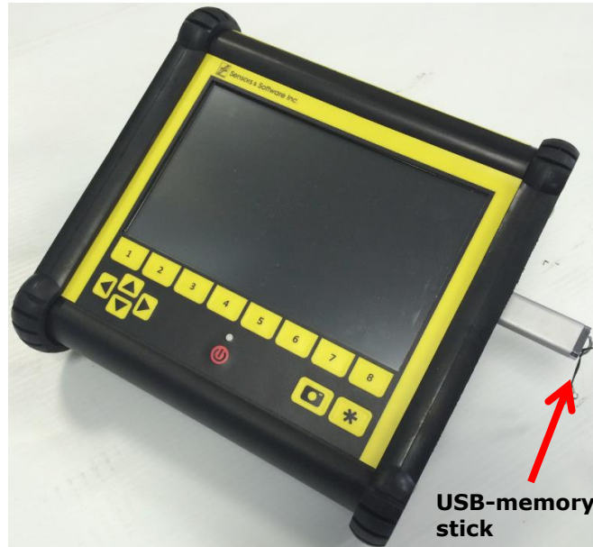
Figure 8-1: Insert a USB memory stick into the USB port on the Display Unit to export data.
