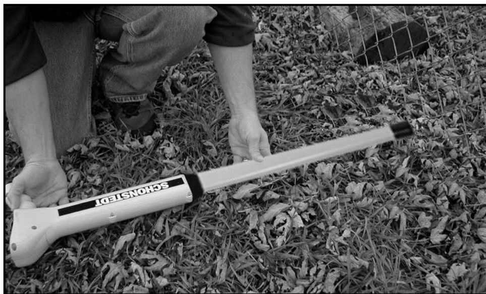
Figure 21: Searching in the Vicinity of a Chain Link Fence
