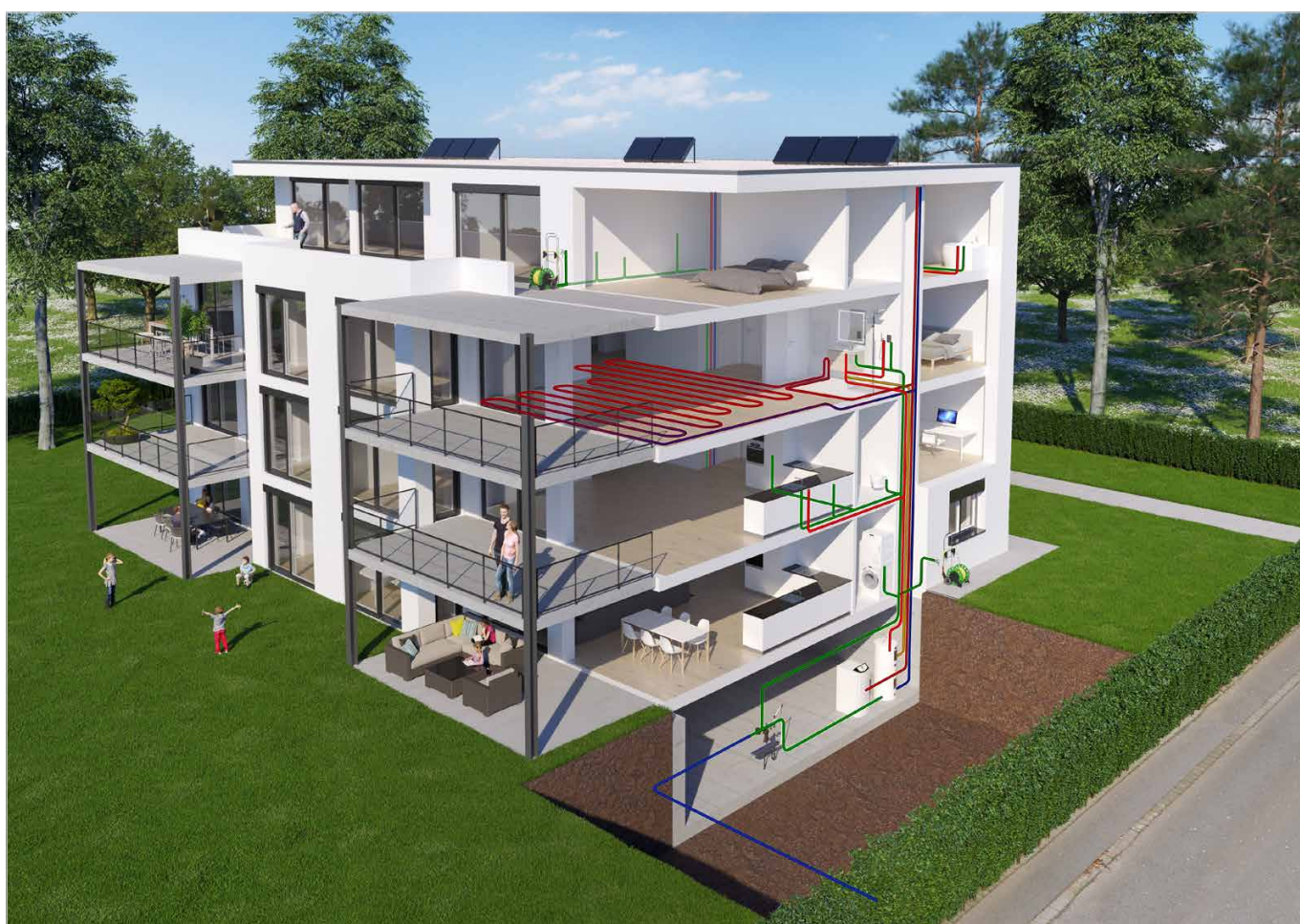
GIV.1 Drinking water installation (exemplary, typical representation)
