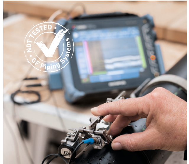
Scan butt fusion welds with our customized ultrasonic sensors
