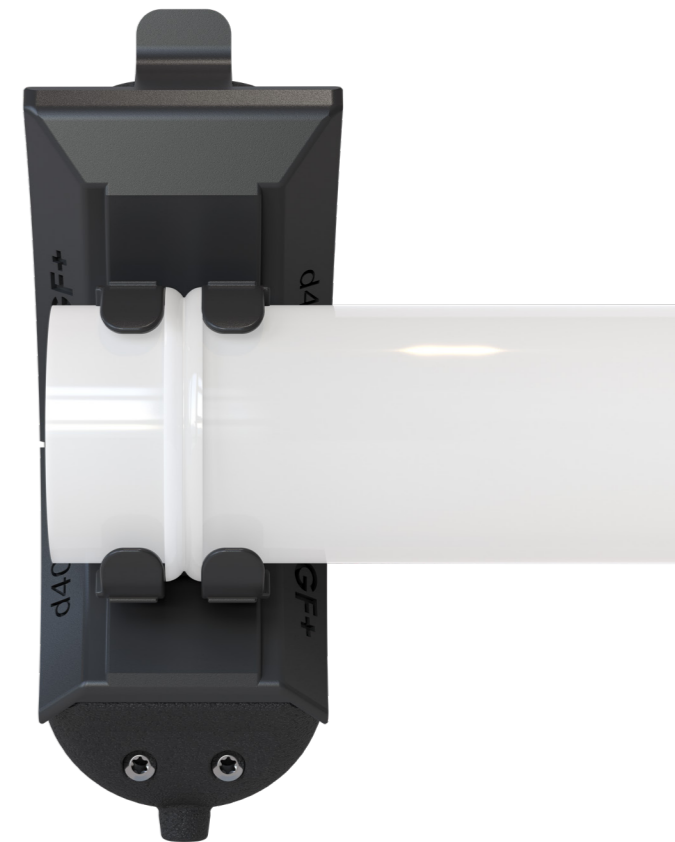
WBI Tool assesses between 4-16 measuring points
